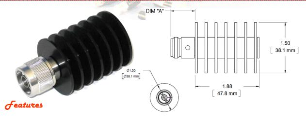
N-type or SMA stainless steel M/F connector per MIL-STD-348A, interface dimensions mate non-destructively with MIL-PRF-39012. Designed to meet MIL-DTL-3933 environmental specification. Unit may be mounted in any position.
