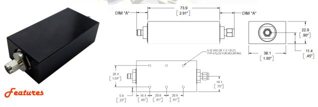
Type N, SMA, or TNC stainless steel M/F connectors per MIL-STD-348A, interface dimensions mate nondestructively with MIL-PRF-39012. Designed to meet MIL-DTL-3933 environmental specification. Flat body with 6-32 mounting holes for conductive cooling.
