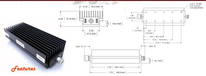
Type N or 7/16 DIN stainless steel connectors per MIL-STD-348A, interface non-destructively with MIL-PRF-39012. Designed to meet MIL-DTL-3933 environmental specification. Passive cooling, flat base with mounting holes.
