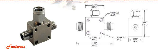
Male 3.5mm port 1, (2) female 3.5mm ports 2 and 3; all ports -mate non-destructively with other SMA, 2.92mm and 3.5mm connectors. Optional female 3.5mm connectors are available on all ports. Designed to meet MIL-DTL-3933 environmental specification.
