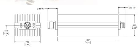
Type N or 7/16 DIN stainless steel connectors per MIL-STD-348A, interface non-destructively with MIL-PRF-39012. Designed to meet MIL-DTL-3933 environmental specification.
