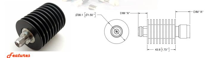
Type N, SMA, or 7/16 DIN stainless steel connectors per MIL-STD-348A, interface nondestructively with MIL-PRF-39012. Designed to meet MIL-DTL-3933 environmental specification.
