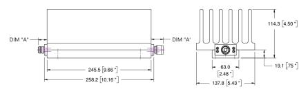
Type N or DIN 7/16 stainless steel M/F connectors per MIL-STD-348A, interface dimensions mate nondestructively with MIL-PRF-39012. Designed to meet MIL-DTL-3933 environmental specification.
