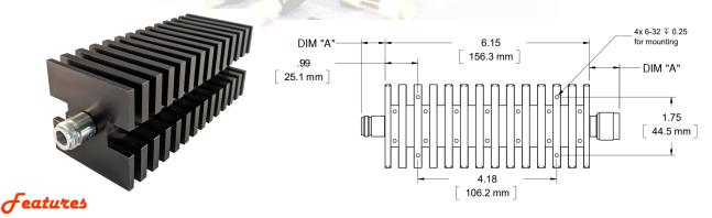
SMA, Type N, and TNC stainless steel M/F connectors per MIL-STD-348A, interface dimensions mate nondestructively with MIL-PRF-39012. Designed to meet MIL-DTL-3933 environmental specification.
