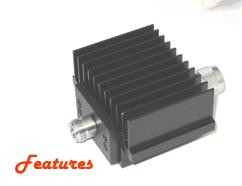
Type N, SMA, TNC, or 7/16 DIN stainless steel connectors per MIL-STD-348A, interface non-destructively with MIL-PRF-39012. Designed to meet MIL-DTL-3933 environmental specification. Passive cooling, flat base with mounting holes.
