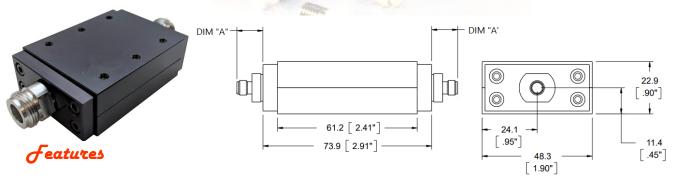
Type N, SMA or TNC stainless steel M/F connectors per MIL-STD-348A, interface dimensions mate nondestructively with MIL-PRF-39012. Designed to meet MIL-DTL-3933 environmental specification. Flat body with 6-32 mounting holes for conductive cooling.
