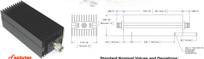
Type N or DIN 7/16 stainless steel M/F connectors per MIL-STD-348A, interface dimensions mate nondestructively with MIL-PRF-39012. Designed to meet MIL-DTL-3933 environmental specification.
