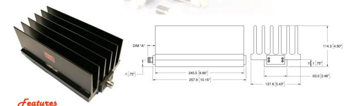
Type N or DIN 7/16 stainless steel M/F connector per MIL-STD-348A, interface dimensions mate nondestructively with MIL-PRF-39012. Designed to meet MIL-DTL-3933 environmental specification. Unit may be mounted in any position.
