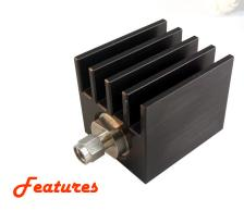
Type N, SMA, or TNC stainless steel connectors per MIL-STD-348A, interface non-destructively with MIL-PRF-39012. Designed to meet MIL-DTL-3933 environmental specification. Passive cooling, flat base with mounting holes.
