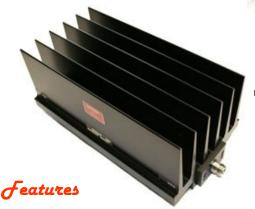
Type N or DIN 7/16 stainless steel M/F connectors per MIL-STD-348A, interface dimensions mate nondestructively with MIL-PRF-39012. Designed to meet MIL-DTL-3933 environmental specification.
