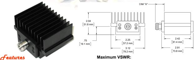
Type N, TNC, SMA or DIN 7/16 stainless steel M/ F connector per MIL-STD-348A, interface dimensions mate nondestructively with MIL-PRF-39012. Designed to meet MIL-DTL-3933 environmental specification. Unit may be mounted in any position.
