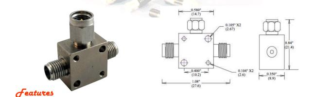
Male precision 2.92 mm port 1, (2) Female precision 2.92 mm ports 2 and 3; all ports-mate nondestructively with other SMA, 2.92mm and 3.5mm connectors. Designed to meet MIL-DTL-3933 environmental specification.
