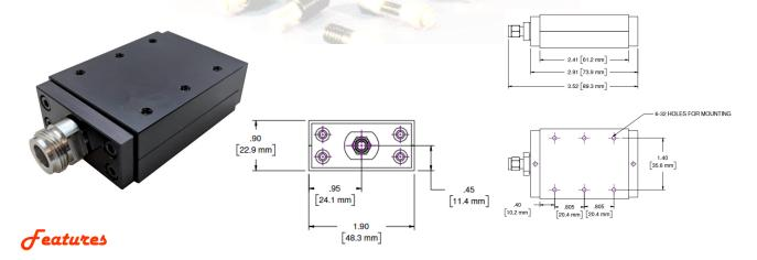
Type N, TNC or SMA stainless steel M/F connecters per MIL-STD-348A, interface dimensions mate non-destructively with MIL-PRF-39012. Designed to meet MIL-DTL-3933 environmental specification. Unit may be mounted in any position.
