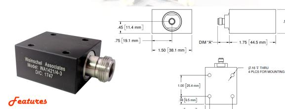
SMA, N-type or TNC stainless steel M/F connector per MIL-STD-348A, interface dimensions mate nondestructively with MIL-PRF-39012. Designed to meet MIL-DTL-3933 environmental specification. Unit may be mounted in any position.
