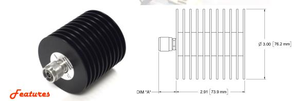
Type N, TNC, SMA or DIN 7/16 stainless steel M/F connector per MIL-STD-348A, interface dimensions mate nondestructively with MIL-PRF-39012. Designed to meet MIL-DTL-3933 environmental specification. Unit may be mounted in any position.
