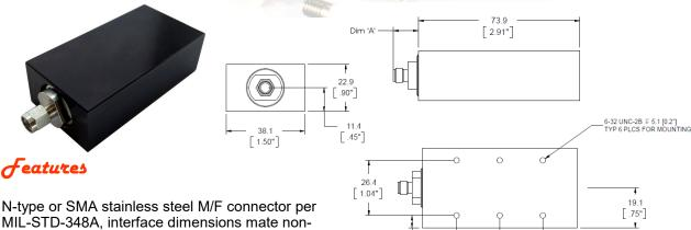
M-type or SMA stainless steel M/F connector per MIL-STD-348A, interface dimensions mate non-destructively with MIL-PRF-39012. Designed to meet MIL-DTL-3933 environmental specification. Unit may be mounted in any position.
