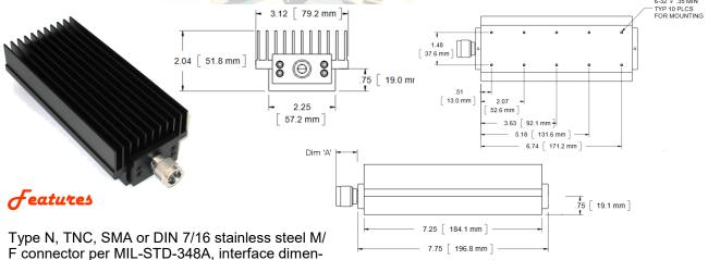
Type N, TNC, SMA or DIN 7/16 stainless steel M F connector per MIL-STD-348A, interface dimensions mate nondestructively with MIL-PRF-39012. Designed to meet MIL-DTL-3933 environmental specification. Unit may be mounted in any position.
